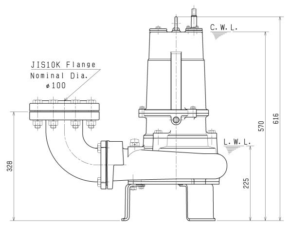
C. W. L. :Continuous runnning Water Level L. W. L. :Lowest runnning Water Level
